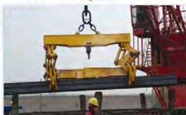
双层钢坯起吊型应用 Double steel billet lifting applications
