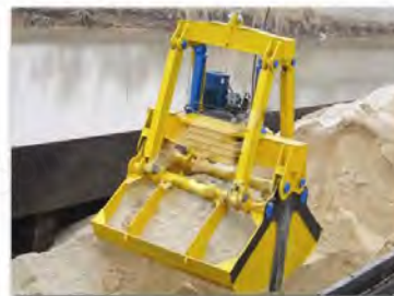
液压抓斗吊装实例 Hydraulic crab bucket hoisting instance
